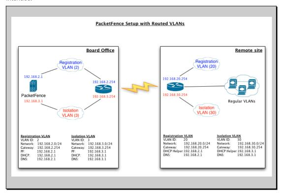
For dhcpd, make sure that the clients DHCP requests are correctly forwarded (IP Helpers in the remote routers) to the PacketFence server. Then make sure you followed the instructions in the <u>DHCP and DNS Server Configuration (networks.conf)</u> for your locally accessible network.
