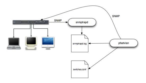
You need to create a registration VLAN (with a DHCP server, but no routing to other VLANs) in which PacketFence will put unregistered devices. If you want to isolate computers which have open violations in a separate VLAN, an isolation VLAN needs also to be created.
