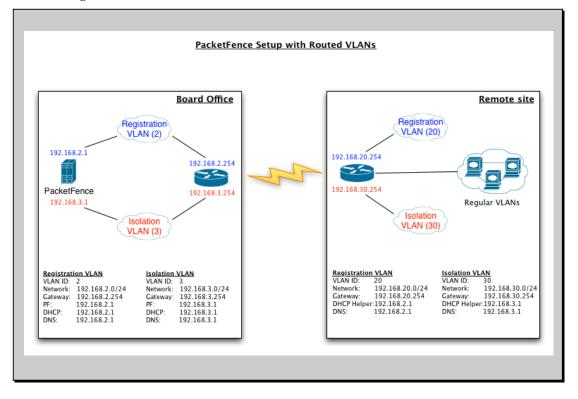
For dhcpd, make sure that the clients DHCP requests are correctly forwarded (IP Helpers in the remote routers) to the PacketFence server. Then make sure you followed the instructions in the DHCP and DNS Server Configuration (networks.conf) for your locally accessible network.
