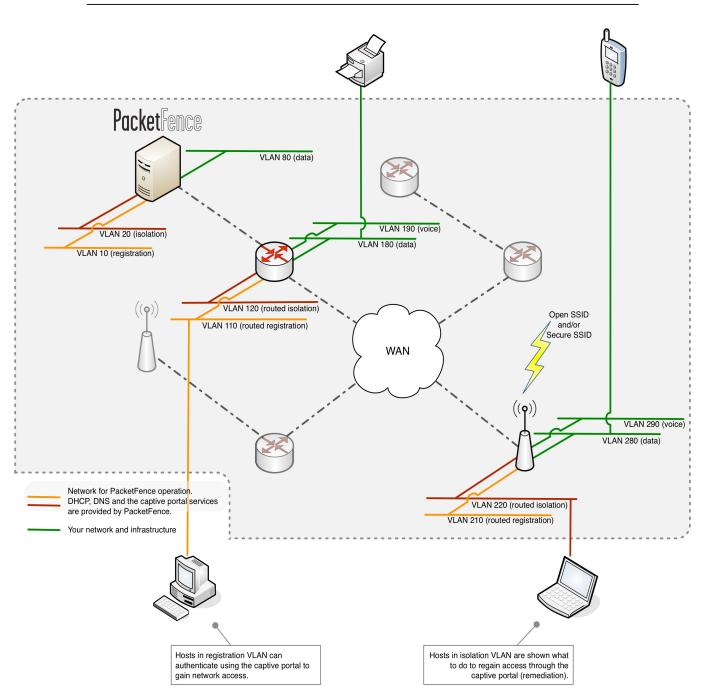
VLAN enforcement is pictured in the above diagram. Inline enforcement should be seen as a simple flat network where PacketFence acts as a firewall / gateway.
