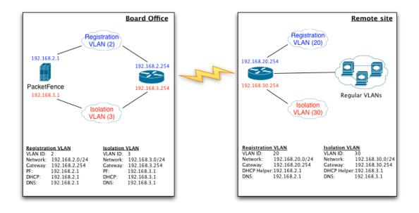
For dhcpd, make sure that the clients DHCP requests are correctly forwarded (IP Helpers in the remote routers) to the PacketFence server. Then make sure you followed the instructions in the <u>DHCP and DNS</u> <u>Server Configuration (networks.conf)</u> for your locally accessible network.
