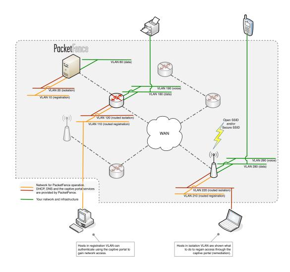
VLAN enforcement is pictured in the above diagram. Inline enforcement should be seen as a simple flat network where PacketFence acts as a firewall / gateway.
