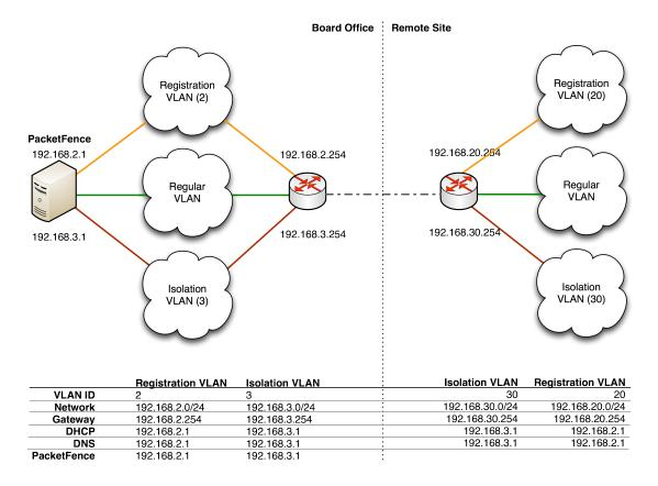
For dhcpd, make sure that the clients DHCP requests are correctly forwarded (IP Helpers in the remote routers) to the PacketFence server. Then make sure you followed the instructions in the <u>DHCP and DNS Server Configuration (networks.conf)</u> for your locally accessible network.
