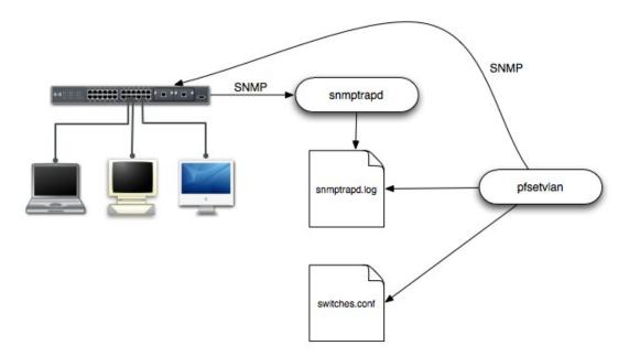
You need to create a registration VLAN (with a DHCP server, but no routing to other VLANs) in which PacketFence will put unregistered devices. If you want to isolate computers which have open violations in a separate VLAN, an isolation VLAN needs also to be created.
