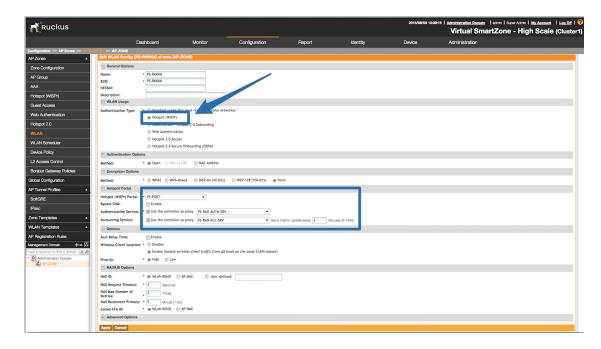
Now, you should configure the Northbound API of the SmartZone so PacketFence can communicate with it. In order to do so, go in *Configuration—System—Northbound Portal Interface* and set the *Password* and save it. Keep the password closeby as it will be required for the PacketFence configuration. In this example, it will be passwordForNorthboundAPI.
